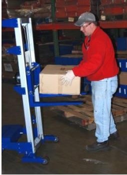
Raise the forks to a comfortable height by turning winch handle clockwise.
