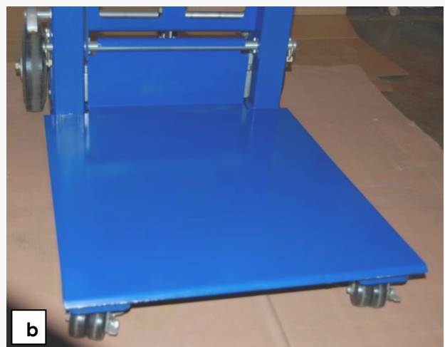
Set the lip on top of the lower carriage cross bar; let the deck rest on top of the forks.
