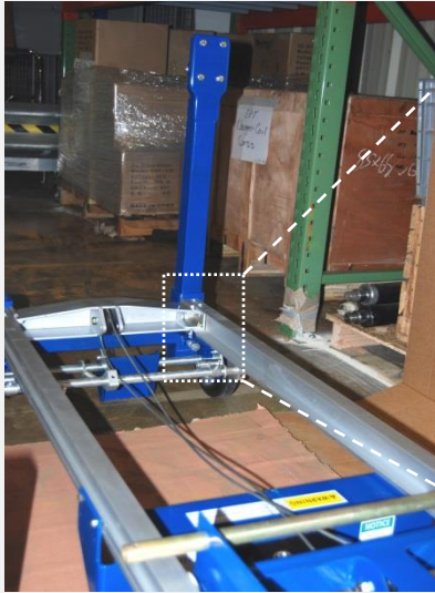
Spring-loaded retaining peg
