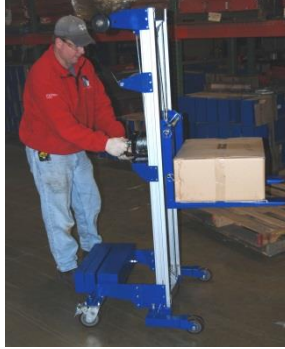
Set the load on the forks. The load must rest against the back of the forks.
