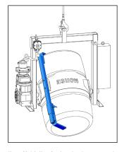
A 55-gallon (210 liter) plastic drum can be handled if the unit is equipped with the adjustable Bracket Assembly (Part # 4556-P). This bracket bolts onto the drum holder, and prevents a 55-gallon (210 liter) plastic drum from slipping lengthways.
