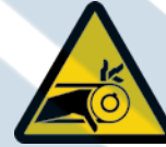
Belt Drive Entanglement Hazard SAX394 SAX395
