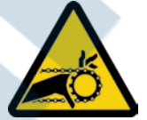
Chain Drive Entanglement Hazard SAX396 SAX397
