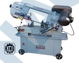
Model No. TS211 Mfg. No. KC-712-BC Cutting capacity at 90°: Rect. 7" x 12", Round 7" Cutting capacity at 45°: Rect. 4-1/2" x 5", Round 5" Speeds: 4 (85, 130, 180, 235 FPM) 0.75" x 0.032" x 93" Blade: Motor: 1 HP, 12 A @ 110 V, 1 phase, 60 Hz Voltage: 110 V Pre-wired at: 110 V **Dimensions:** 50" L x 20" W x 39" H Weight: 275 lbs. Price/Each \$
