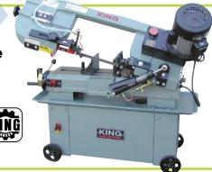
Model No. BV709 Mfg. No. KC-712GH-5 Cutting capacity at 90°: Rect. 7" x 12", Round 7" Cutting capacity at 45°: Rect. 4-1/2" x 5", Round 5" 3 (110, 230, 340 FPM) Speeds: Blade: 0.75" x 0.032" x 93" Motor: 1 HP, 14 A, 1 phase, 60 Hz Voltage: 110 V **Dimensions:** 47" L x 21" W x 40" H 280 lbs. Weight:
